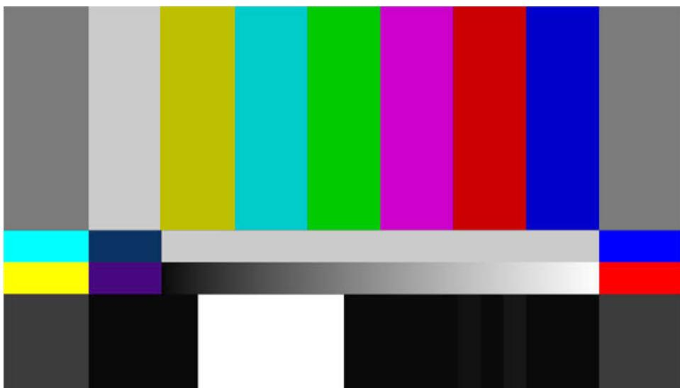
Correct use of these test signals will help you set your monitor's brightness, contrast, and chroma levels. You can use either one of these interchangeably and one is not necessarily more accurate than the other. The process of using either of these color fields is virtually identical.
